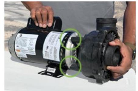
**4** At the back of the motor, push through bolts in until they touch the wet end.
