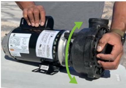
**3** Once in the general location, line up the female threading of the brass inserts on the wet end with the through bolts.
