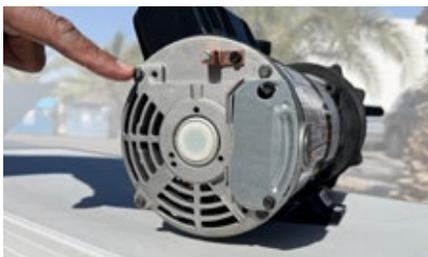
**5** Use a nut driver or socket wrench to screw them back into the wet end.
